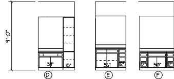
CABINET ELEVATIONS SCALE 1/4" = 1'-0"
