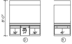
CABINET ELEVATIONS SCALE 1/4" = 1'-0"
